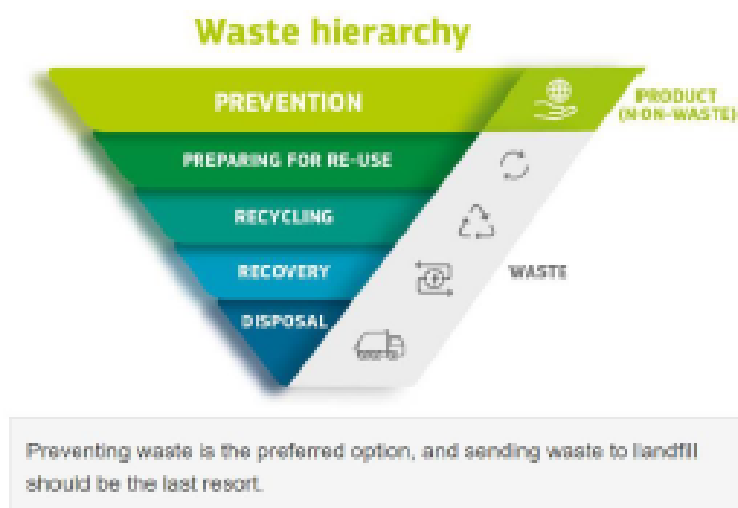
Figure 2: Waste Framework Directive - five step waste hierarchy 1
